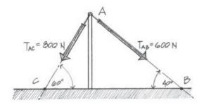
**2.10** Two cables with known tensions as shown are attached to a pole at point A. Determine the resultant force to which the pole is subjected. Scale: 1 mm = 10 N.
