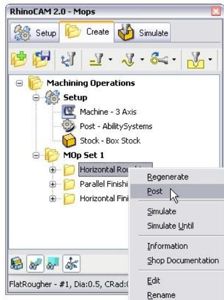
Posting a machining operation
