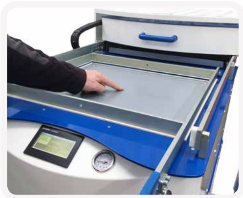
Place your finger over the vacuum hole and check the reading you get on the vacuu gauge.
