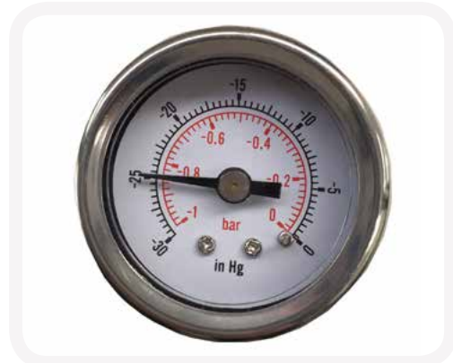
If the vacuum gauge reading of 22”Hg or higher is normal. A lower reading indicated poor vacuum where attention is required.
