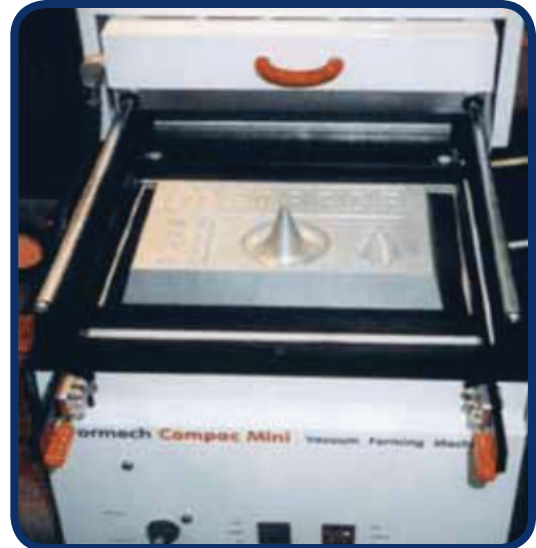
A metaphor mould demonstrated on one of the Formech range of vacuum forming machines
