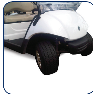
Formech 1500 - Golf Car Parts Acrylic Capped ABS
