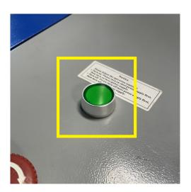
Before you collect your work piece and open the lid make sure to deactivate the laser using the green button.
