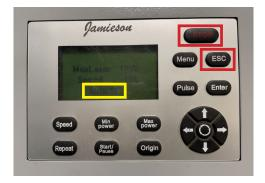
While the file is running, you can see the timer on the control screen. You can also click the STOP button to pause the file and the ESC button to end the file early if needed.
