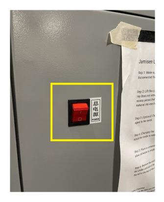
This will turn on the laser cutter as well as turn on the water chiller located next to the machine. If the chiller does not turn on, ask for help.
