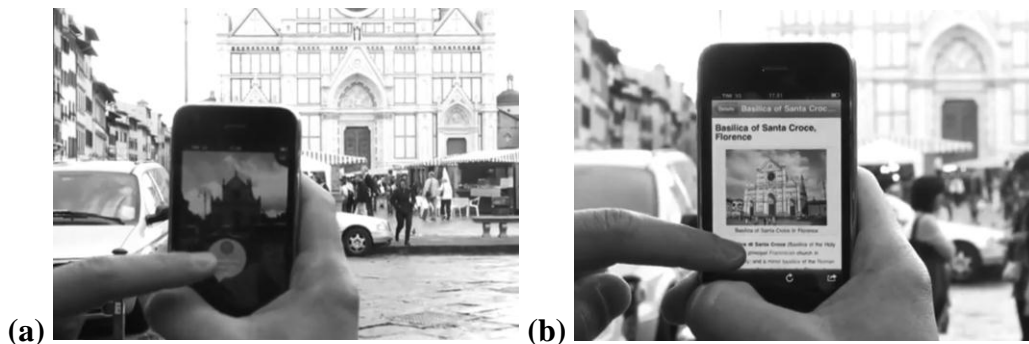
Fig 2. Smart phones allow for location-based AR information to be displayed by (a) pointing at a historic structure having it identified with an icon on the screen. By touching the icon (b), web-based information about the place is displayed.
