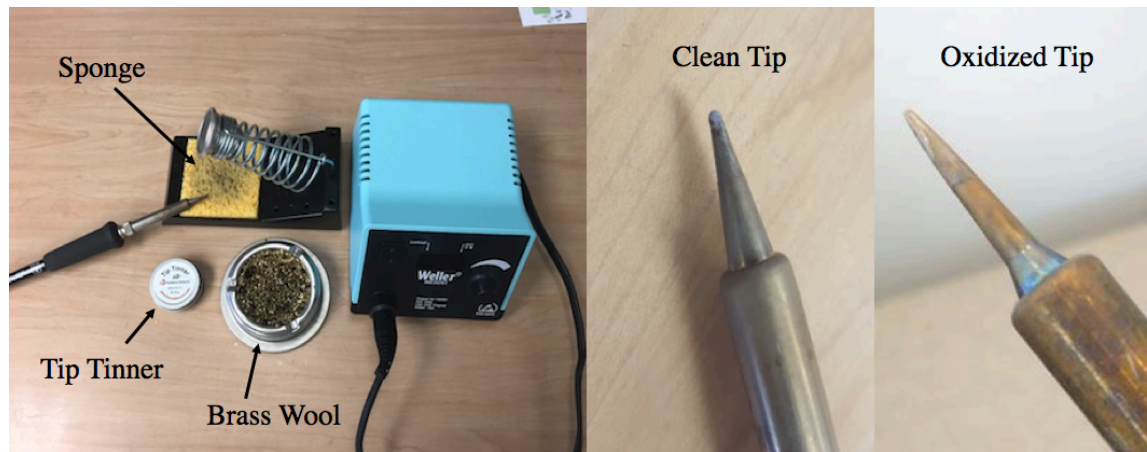
Figure 21. Tools used to protect the iron's tip: a wet sponge, tip tinner, and brass wool. Also, comparison between a clean tip and an oxidized tip.
