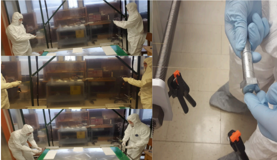
Figure 19. Several key steps in manipulating a wire segment using the transport bolts: transfer the wire to the bolts and gently tension, translate the wire over the MWPC, lower the wire into position.
