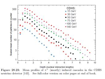
Figure 32: Mean profiles of  $\pi^+$  induced cascades in the CDHS neutrino detector.
