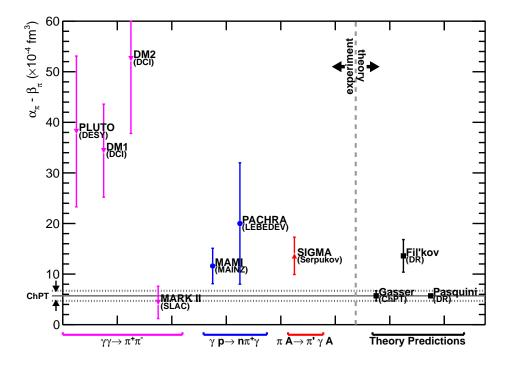
Figure 1: Experimental data for  $\alpha_{\pi} - \beta_{\pi}$  grouped by experiment type, and theoretical predictions
