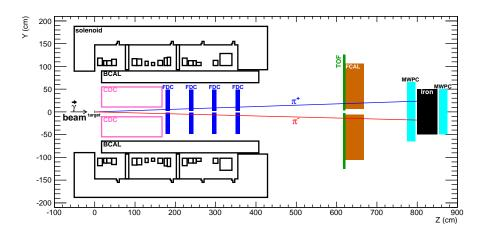
Figure 17: Diagram of the GlueX detector
