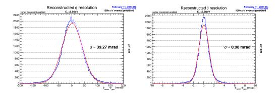
Figure 20: Reconstructed angular resolutions for single tracks. The red curves are from Gaussian fits to the blue distributions.
