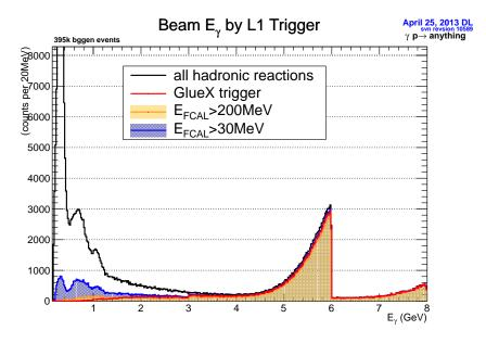
Figure 23: Level-1 trigger selection of incident photon energies. The  $E_{FCAL} > 30 MeV$  trigger accepts about 45% of all hadronic interaction events with a bias towards higher energies.
