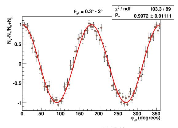
Figure 27: The function  $P_{\gamma} \cos 2\varphi$  fitted to the ratio  $\frac{N_v(\varphi) - N_h(\varphi)}{N_v(\varphi) + N_h(\varphi)}$  with  $P_{\gamma}$  as the free parameter.
