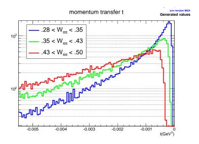
Figure 12: Histogram of t for Primakoff and  $\rho^0$  events. The blue curve is for events with  $0.28 < W_{\pi\pi} < 0.35$  GeV, green is for events with  $0.35 < W_{\pi\pi} < 0.43$  GeV, and red is for events with  $0.43 < W_{\pi\pi} < 0.50$  GeV.
