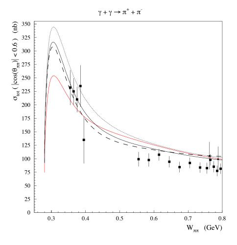
Figure 2:  $\gamma \gamma \rightarrow \pi^+ \pi^-$  cross sections. Red curve: Born approx. (no polarizability effect); black solid: unsubtracted DR calculation with  $\alpha_{\pi} - \beta_{\pi} = 5.7$ ; dashed: subtracted DR with  $\alpha_{\pi} - \beta_{\pi} = 5.7$ ; dotted: subtracted DR with  $\alpha_{\pi} - \beta_{\pi} = 13.0$ . Data points are from MARK-II
