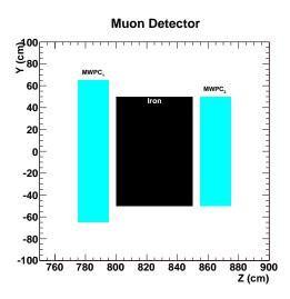
Figure 31: Sketch of muon detector, consisting of a passive iron shield sandwiched between two sets of multi-wire proportional chambers,  $MWPC_1$  and  $MWPC_2$ . The optimal transverse dimensions of the chambers are still being evaluated.
