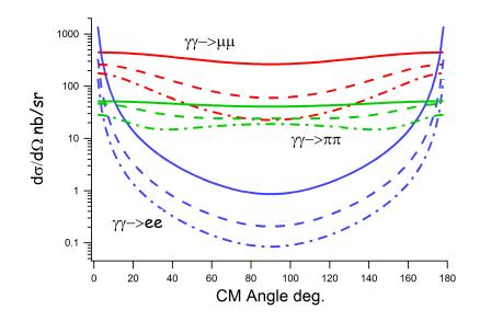
Figure 16: Angular distributions for  $e^+e^-$ ,  $\mu^+\mu^-$  and  $\pi^+\pi^-$  pairs are shown as red, green and blue curves, respectively. The solid, dashed, and dash-dot curves are for 300, 400 and 500 MeV CM energies.
