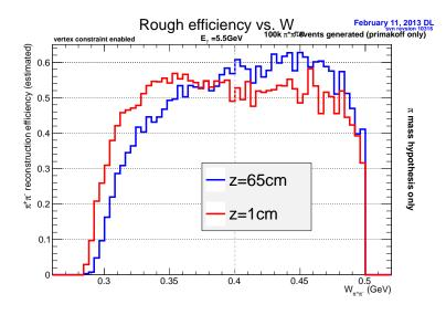
Figure 19: Acceptance of  $\pi^+\pi^-$  events for locating the Pb target at the nominal location of the center of the GlueX target (z=65 cm) and the location being considered for the current measurement 64 cm upstream at z=1.
