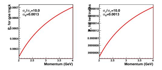
Figure 34: Probability that an event is a pion event, when the muon detector tags one particle as a pion (left plot), and when the muon detector tags both tracks as pions (right plot). The prior probabilities for the pion and muon are assumed to be proportional to their cross sections, where the muon cross section is a factor of ten larger than for pion production.
