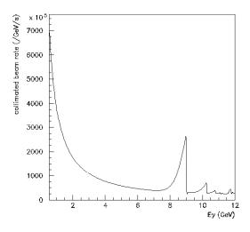
Figure 5: Collimated beam rate at 9 GeV. The ratio of events in the peak (8–9 GeV) to events outside the peak is 0.068.
