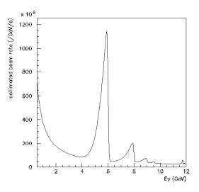
Figure 6: Collimated beam rate at 6 GeV. The ratio of events in the peak (5–6 GeV) to events outside the peak is 0.32.
