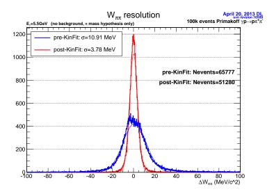
Figure 22: Reconstructed invariant mass  $W_{\pi^+\pi^-}$ . The blue is before a 4C kinematic fit is performed and the red is after.
