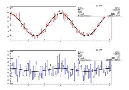
Figure 28: Example fits of the  $\phi_{\pi\pi}$  spectrum (top, red) and the  $\psi_{\pi\pi}$  spectrum (bottom, blue) for the  $W_{\pi\pi}$  bin centered at  $330 MeV/c^2$ . The polarization was fixed at 70% (corresponding to the generated data set). The one free parameter of the fit gave either the fraction of Primakoff (top) or  $\rho^o$  (bottom) events. The angles used here are from generated values, but with a cut on  $\theta > 0.8^\circ$  to represent the acceptance of the detector.
