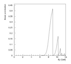
Figure 3: Polarization with peak at 9 GeV. The peak polarization is 44%.
