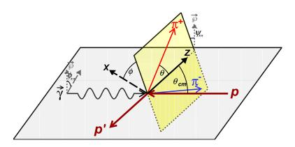
Figure 9: Diagram of the helicity frame for two pion photo-production on the nucleon
