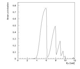
Figure 4: Polarization with peak at 6 GeV. The peak polarization is 76%.
