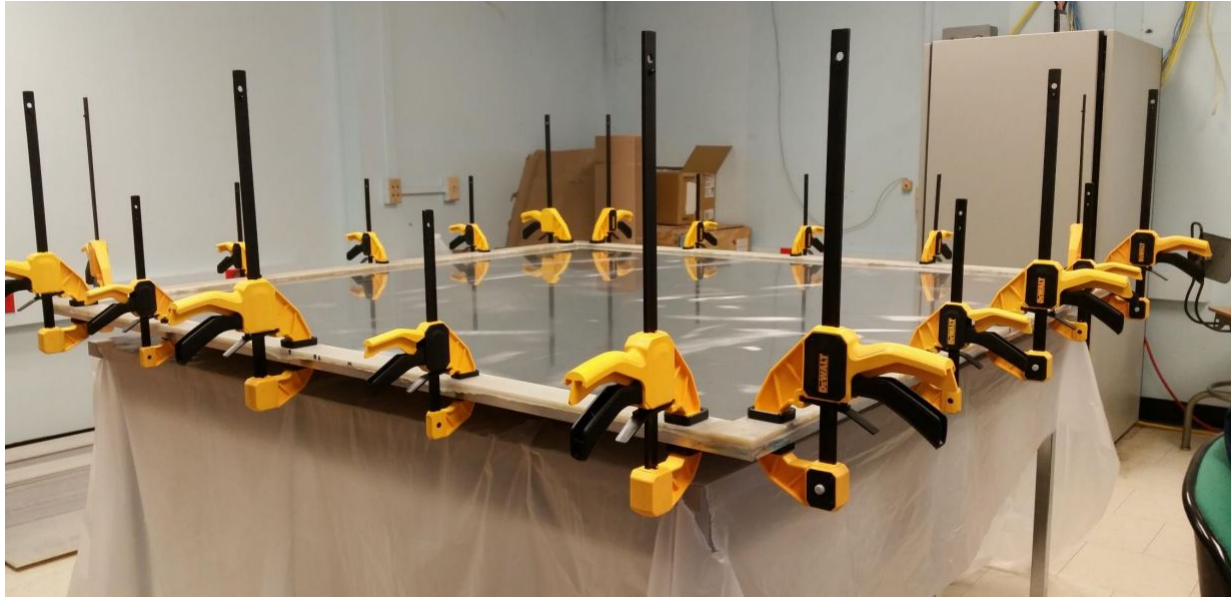
Figure 23: Aluminum plates and G10 plastic slats being epoxied together with the aid of clamps.
