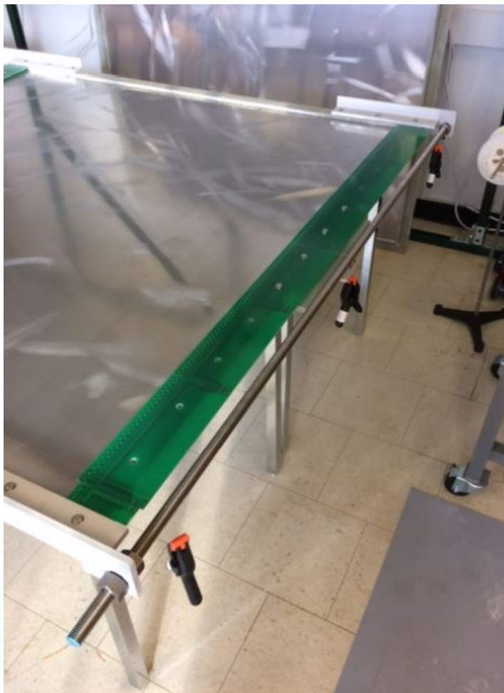
Figure 28: View of detector stringing with positioning wires in place (left, center, and right most pads).
