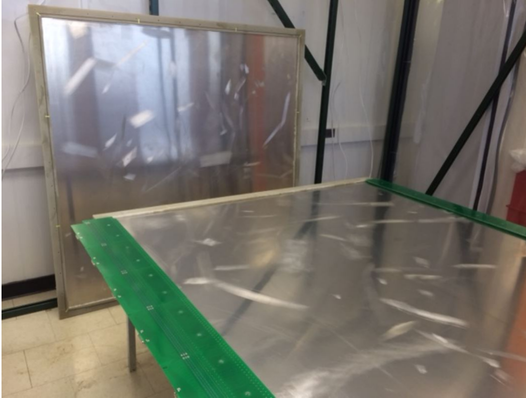
Figure 26: Detector plates with PCBs epoxied to G10 slats.
