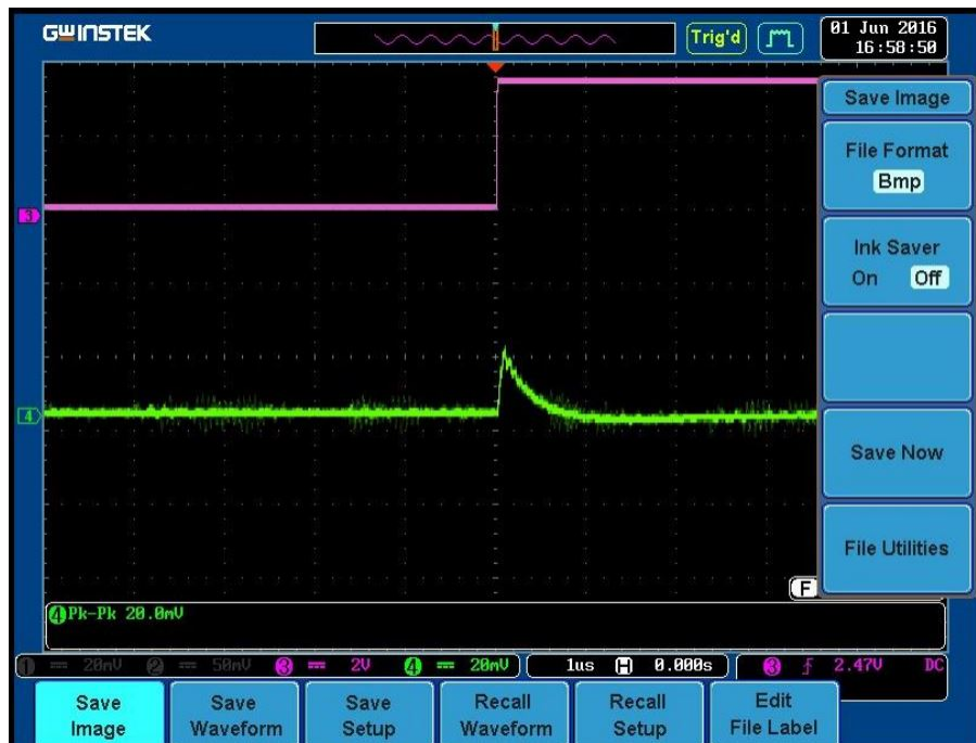
Figure 8: Example oscilloscope output from PCB transformers when testing boards using pulse scope driven with 1 Volt square wave at 50 % duty.
