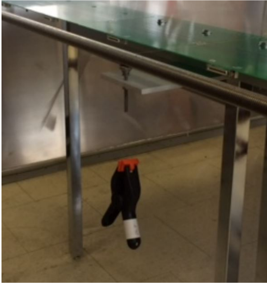
Figure 27: View of detector stringing with ACME rod and support structure in center top of image. Hanging from a non-visible wire is a clamp used to provide tension.
