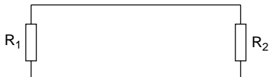
Fig. 6.33 Nyquist's idealized arrangement of two resistors in thermal equilibrium, connected by a lossless transmission line that has no thermal properties
