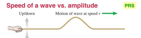
How does the speed with which the wave propagates along the string change when it is shaken more vigorously?
