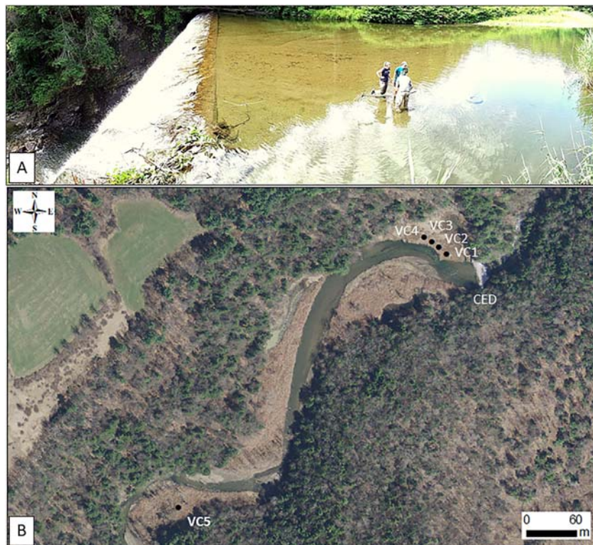
FIGURE 4. (A) Photograph of researchers standing on impounded sediment in the channel just upstream of the Conway Electric Dam (CED), which is on the left side of image. (B) A 2014 aerial orthophotograph of the CED impoundment (30 cm resolution; from MassGIS) and vibracore locations at this site. [Colour figure can be viewed at wileyonlinelibrary.com ]
